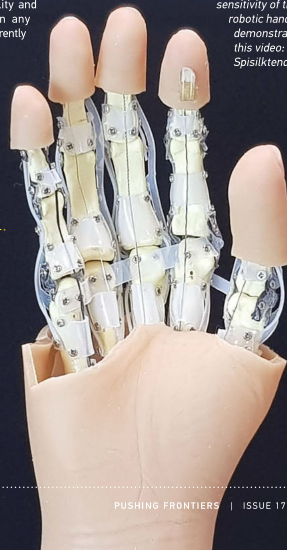
A 3D-printed humanoid robotic hand incorporating an electro-tendon made of spider silk and a pressure sensor mounted on the index finger. Credit: Pan Liang/Chen Xiaodong.
