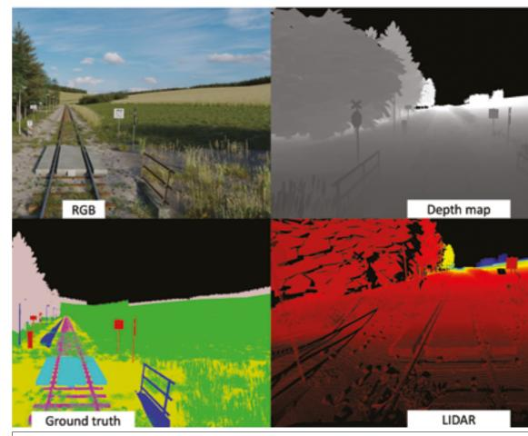
↔ Simulator of train track conditions to improve obstacle detection in real traffic
