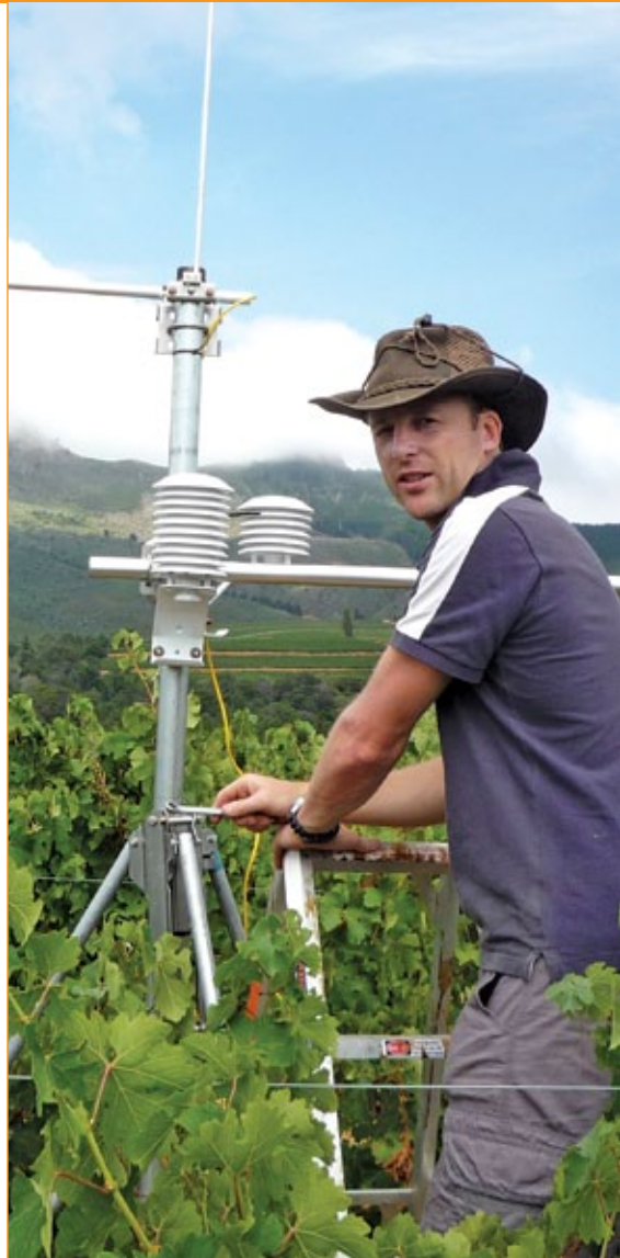
Alistair Clulow, a member of the Centre for Water Resources Research and lecturer in AgMet installing an Eddy Covariance system to measure evaporation from a vineyard as part of a project to test remote sensing approaches to estimate water use and improve irrigation scheduling for different crops.
